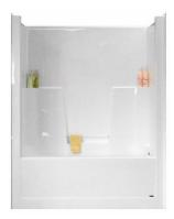
Warm Rain models WR 144-D (right hand) and WR 145-D (left hand) tub/shower fixtures are constructed of reinforced polyester resin covered with a high gloss gel-coat of 18 - 20 mil. thickness. The reinforced fiberglass has a minimum content of 18 % fiberglass.
