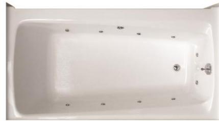
Warm Rain models WR 330AT (right hand plumbing) and WR 331AT (left hand plumbing) Front-Fit™ remodeling tub/shower AirTubs are constructed of reinforced polyester resin covered with a high gloss gel-coat of 18 - 20 mil. thickness. The reinforced fiberglass has a minimum content of 18 % fiberglass. The bottom base of the unit is constructed of 1/2" end-grained balsa wood sandwiched between 2 layers of reinforced. The base is an integral part of the unit.
